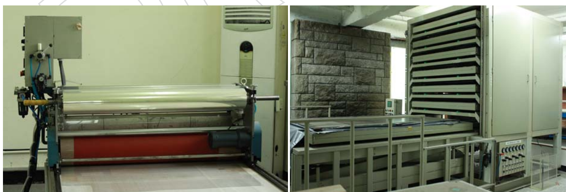
Figure 3.21: a) Electrode insulation machine; b) Gas assembly machine.
