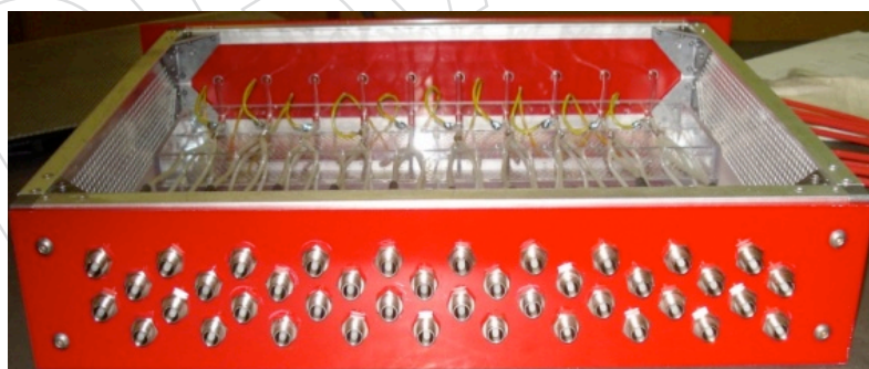
Figure 3.19: HV Distribution board.
