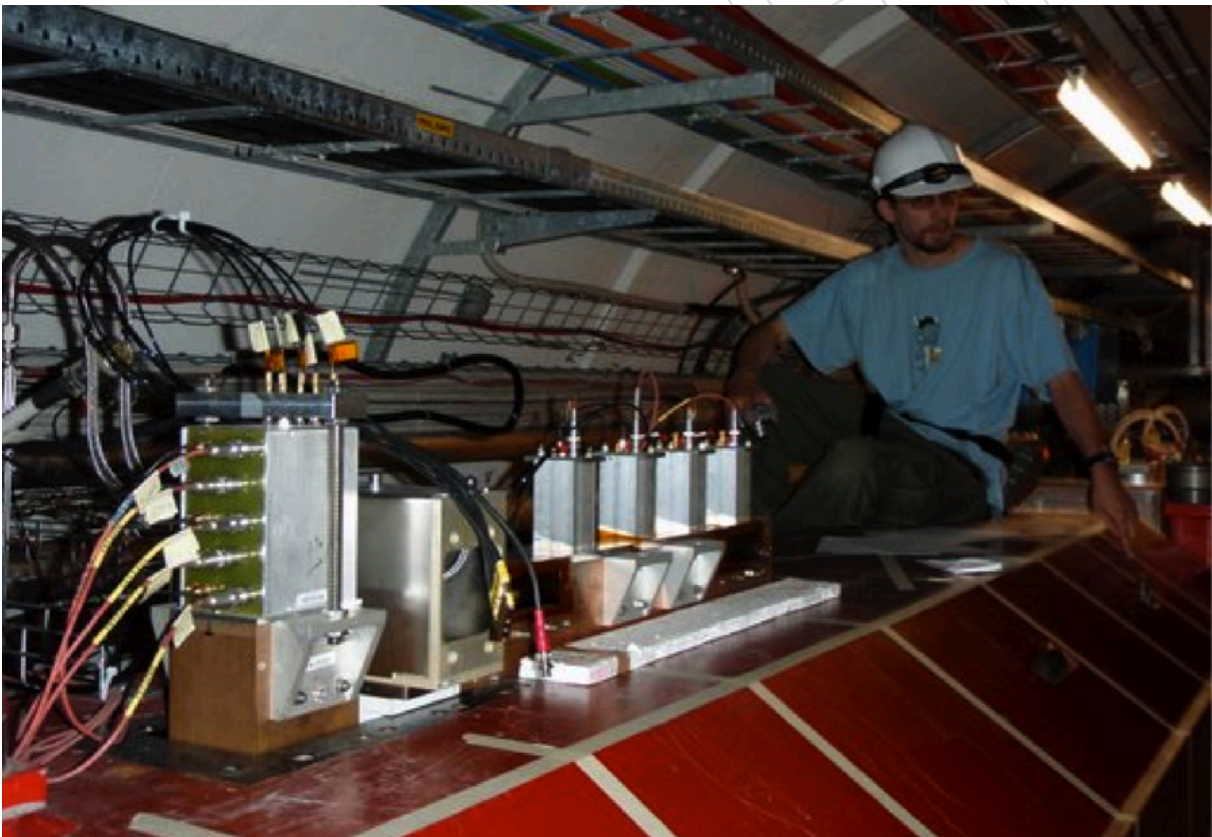
Figure D.1: A photograph of ZDC- in the the TAN absorber. The CMS interaction region is 140m to the left of the detector.
