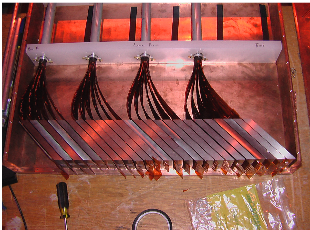
Figure D.3: Photograph of the ZDC HAD section during construction showing the gray tungsten plates, the sheets of quartz fibers and the light guides. The lead/boronated polyethylene shield that lies above the tungsten plates was not yet installed.
