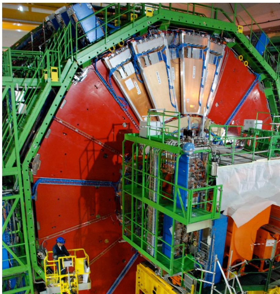
Figure 3.28: 5 ME4/2 chambers installed on the back side of the YE+3 disk.
