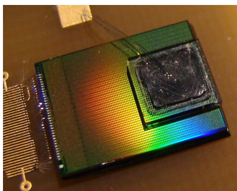
Figure 9.15: Bump bonded detector.
