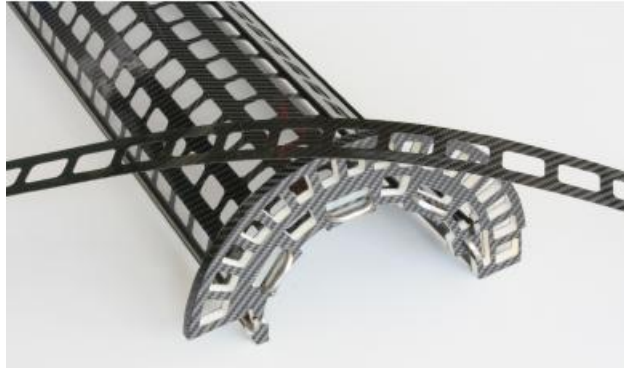
Figure 6.12: Prototype of the mechanical structure for the innermost layer. To illustrate its light-weight, a carbon fiber ladder is laid upon the half-barrel. The mechanical stability of the ladder is given by the cooling tubes.
