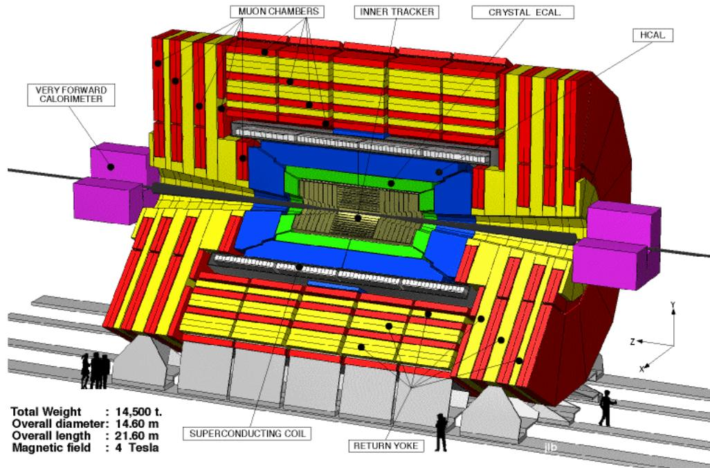
Figure 2.2: Sectional view of the CMS detector with the coordinate axes [2]
