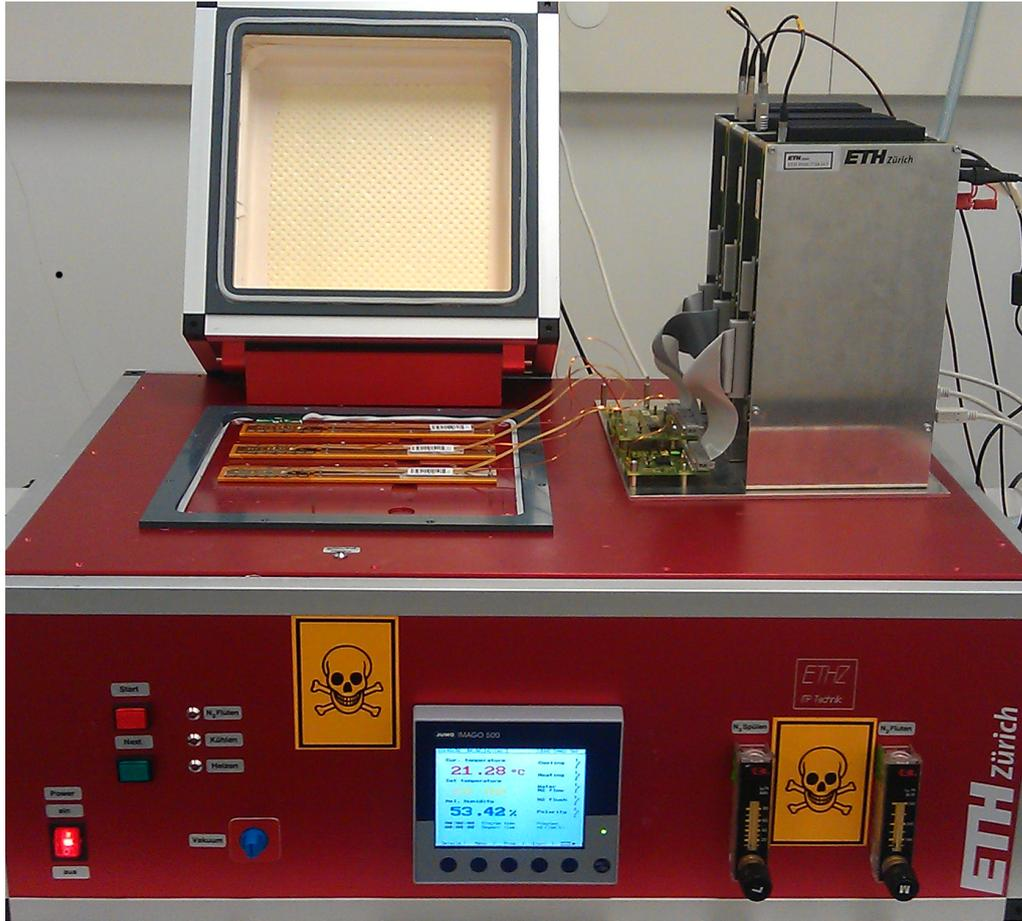
Figure 4.2: The coldbox with three modules, module adapters and testboards.
