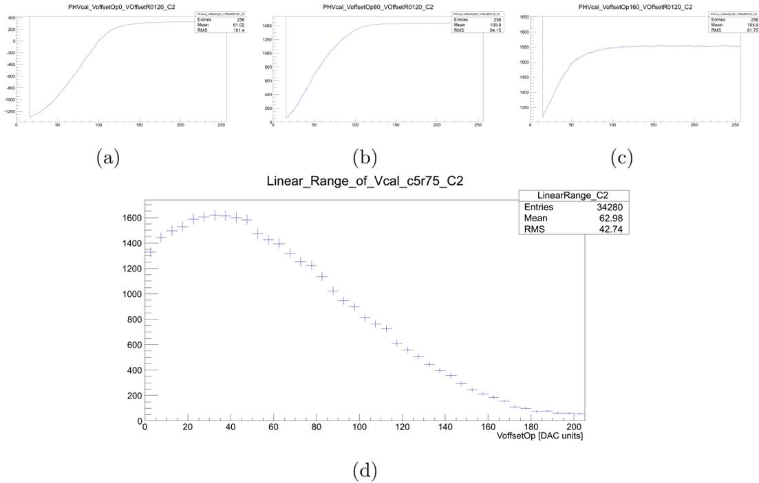
Figure 4.6: VOffsetOp optimization procedure: (a)-(c) The linear range is obtained from a fit for different values of VOffsetOp, three examples are shown for VOffsetOp = 0; 80; 160. (d) The linear range is then plotted as function of VOffsetOp and the position of the maximum linear range is chosen as the optimum value for VOffsetOp.
