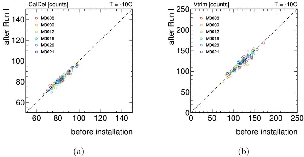
Figure 4.3: The comparison of the tuned DAC parameters from the data of 2008 and 2014. CalDel and Vtrim are on average unchanged.
