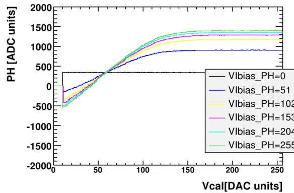
Figure 4.7: The behavior of the pulse height curve for different values of Vbias\_PH [5].
