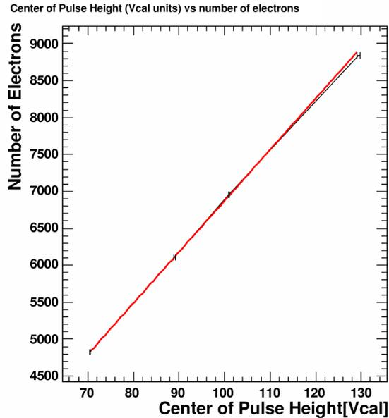
Figure 6.3: The linear fit (red line) to the four target mean positions for ROC3 of M0018
