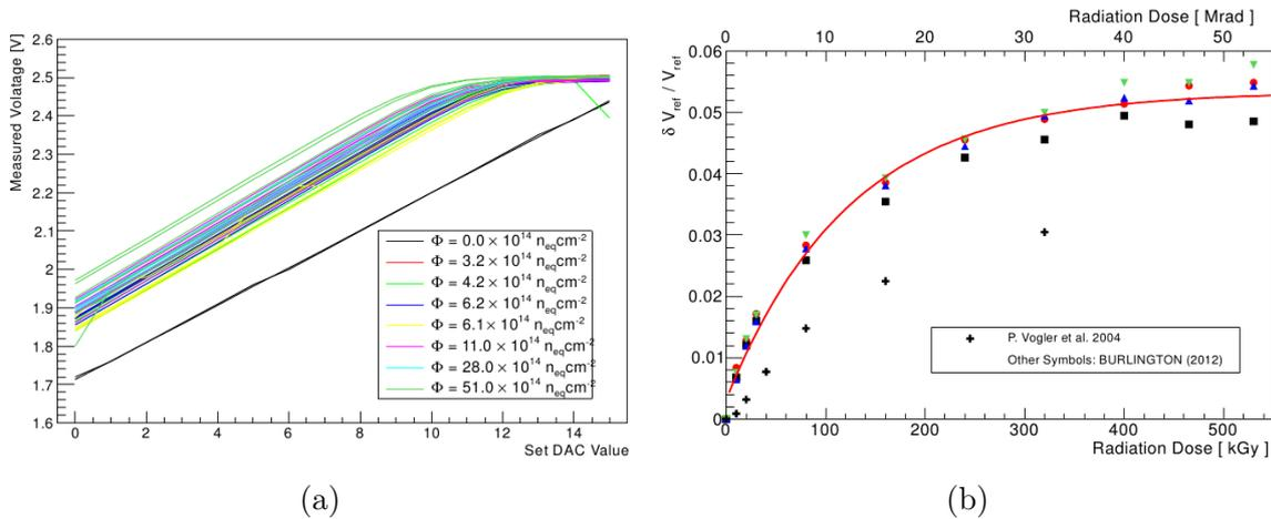
Figure 4.1: (a) shows the linear behavior of the DAC value versus the DAC voltage [9]. (b) shows the expected change in the reference voltage due to radiation [10]
