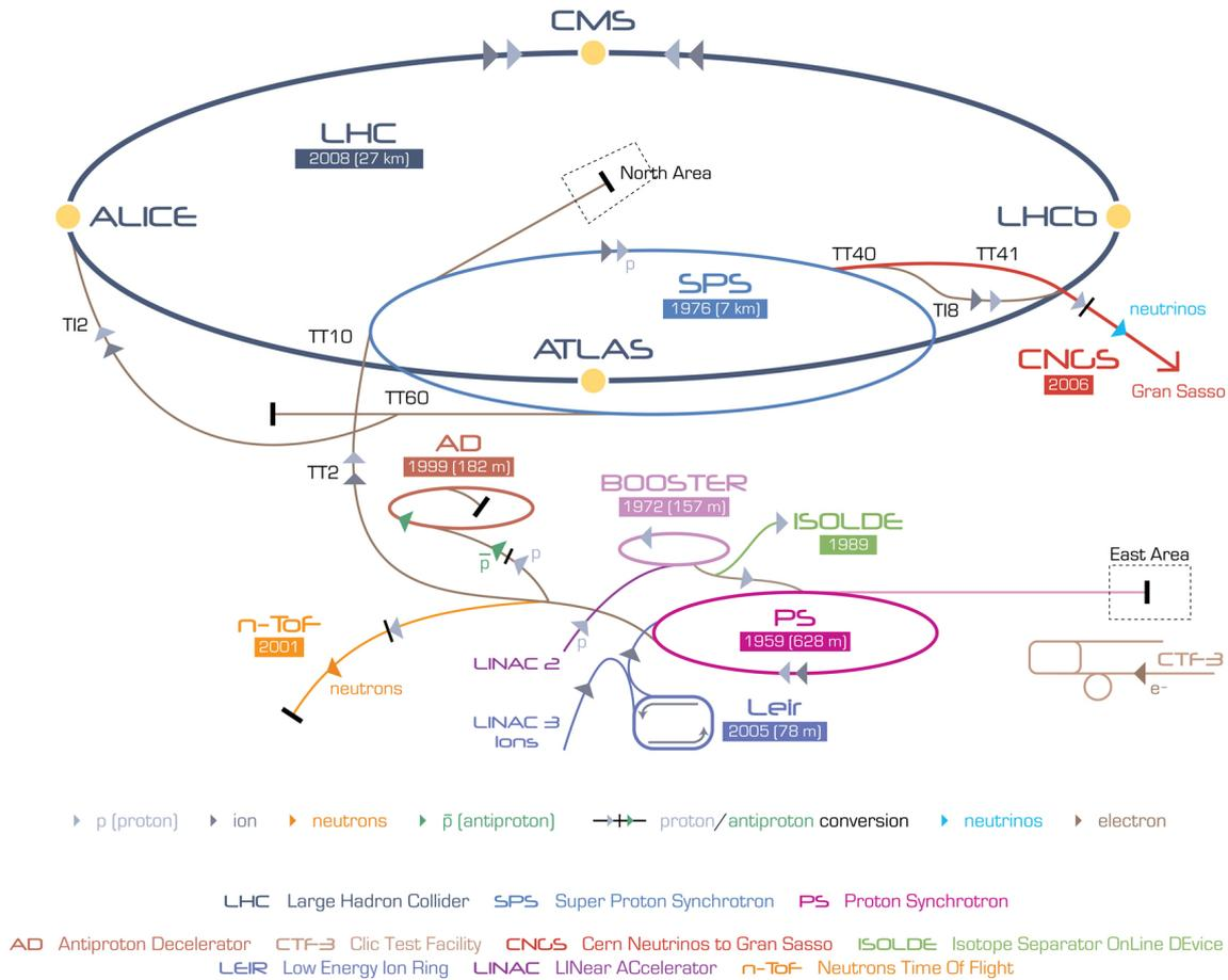
Figure 2.1: The accelerator complex of CERN with the sites of the four detectors [1]
