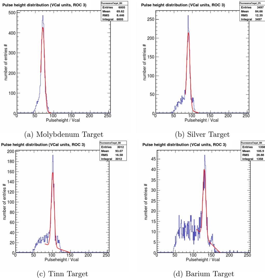
Figure 6.2: The pulse height distributions for the different targets for ROC3 of M0018
