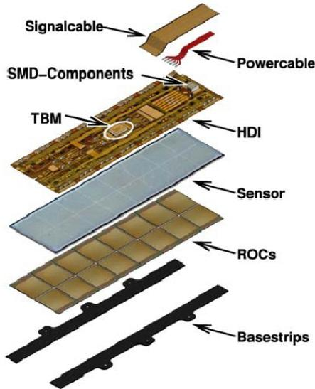
Figure 3.1: Exploded view of a module [4]
