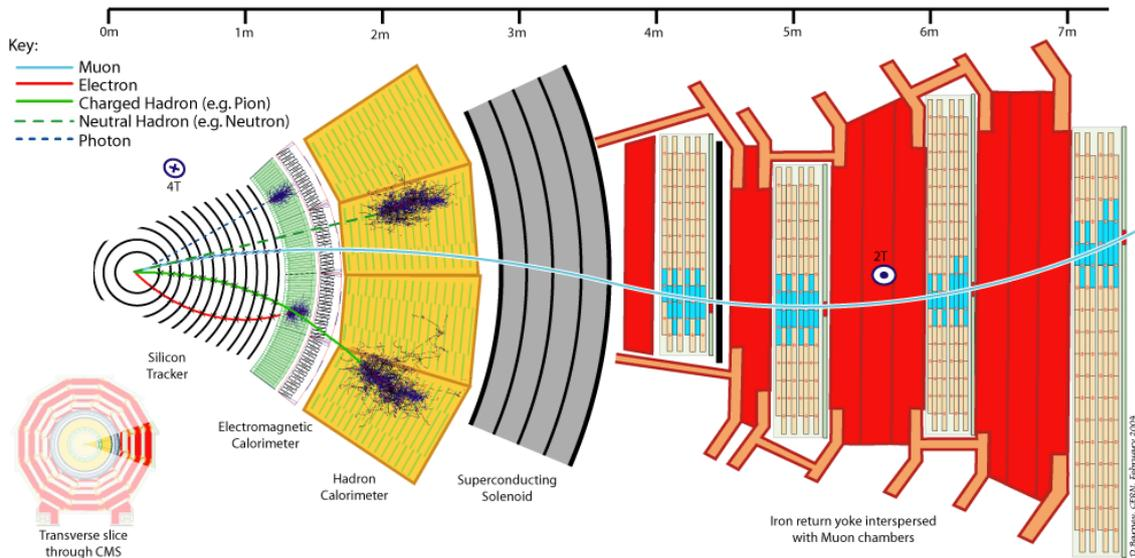
Figure 2.3: The barrel layout of CMS with the track and energy depositions of the different particles in the different detector types [2]
