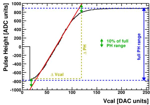
Figure 4.5: Pulse height curve [5]
