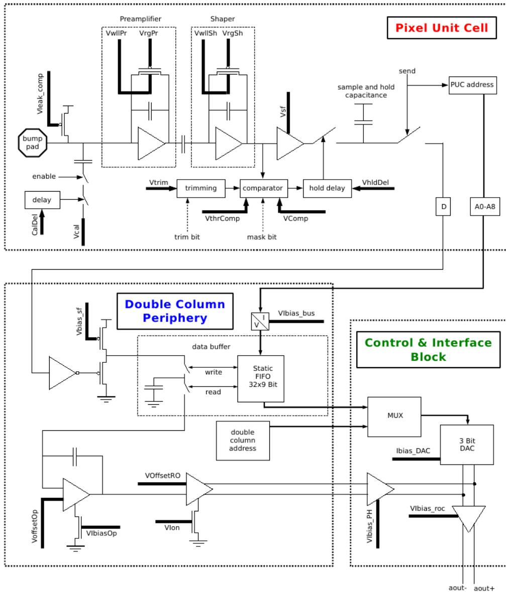
Figure 3.2: Scheme of the pixel unit cell (PUC), the double column periphery and the control & interface block [5]
