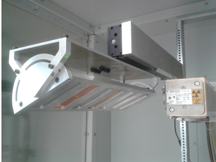
Figure 9: Picture of the X-ray source on the right and the target holder with the seven different target materials on the left. The target holder can be moved such that every target material can be placed in front of the X-ray source.
