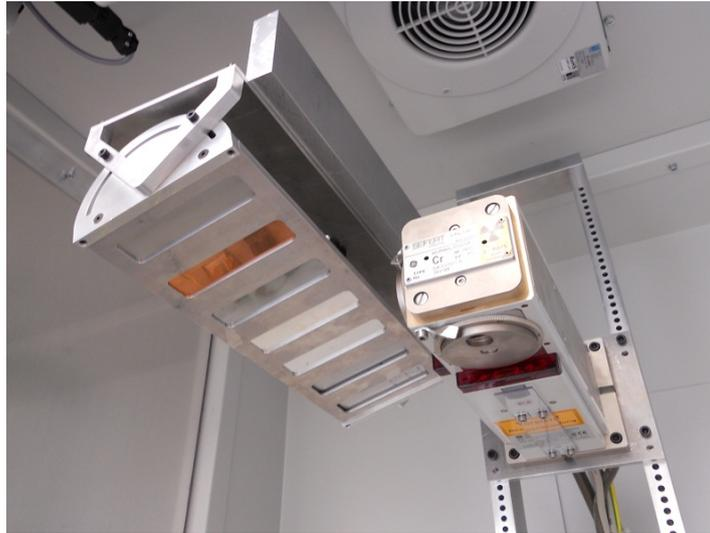
Figure 3.2: Left: Target Array. Right: X-ray tube.
