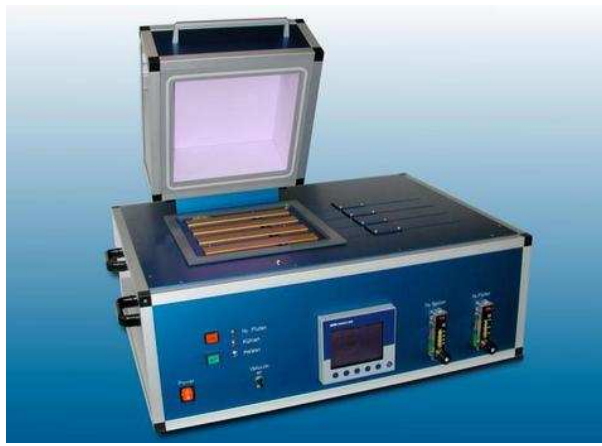
Figure 19: A set-up for thermal test of CMS pixel barrel modules.
